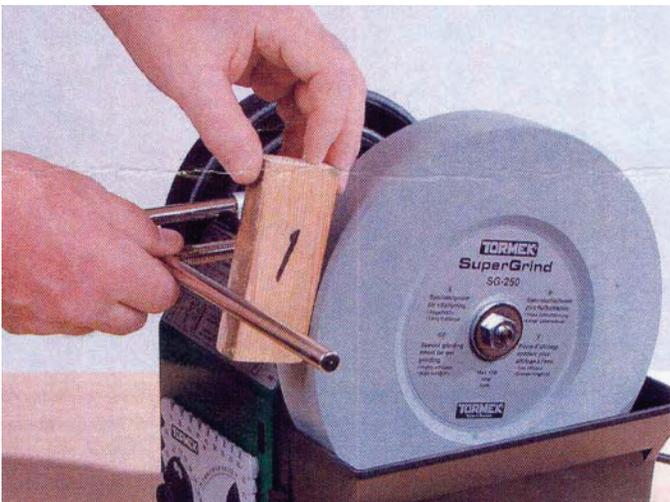
**Take your IR Block and set the Universal Support that thickness (2.05") from the grinding wheel.**
